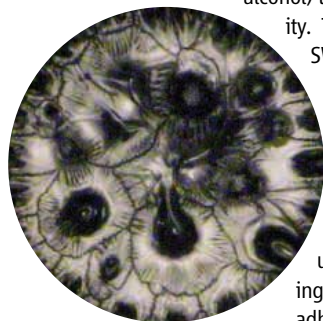
Debonded adhesive surface.
